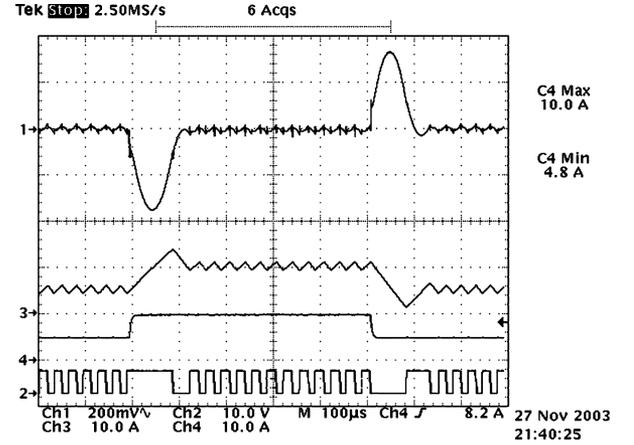
Fig. 9. Transient response of buck converter using second-order switching surface control. Load change from  $5 \text{ A}$  ( $2.4 \Omega$ ) to  $10 \text{ A}$  ( $1.2 \Omega$ ) and vice versa. [Ch1:  $v_C$  ( $200 \text{ mV/div}$ ), Ch2:  $v_g$  ( $10 \text{ V/div}$ ), Ch3:  $i_L$  ( $10 \text{ A/div}$ ), Ch4:  $i_o$  ( $10 \text{ A/div}$ )] (Timebase:  $100 \mu\text{s/div}$ .)
