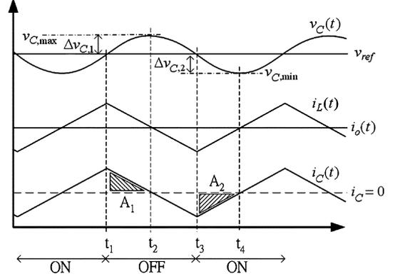
Fig. 3. Typical waveforms of  $v_C$ ,  $i_L$ ,  $i_C$ , and  $i_o$  of buck converter.
