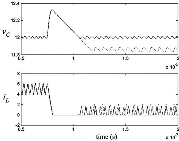
Fig. 8. Transient response of  $R$  from  $2.4$  to  $24 \Omega$ . (Solid line:  $\sigma^2$ , dotted line:  $\sigma^1$ ).
