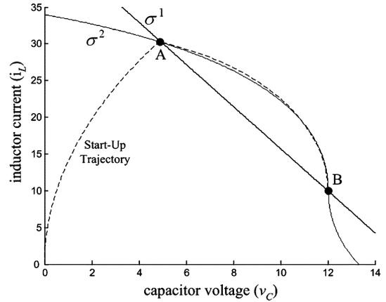
Fig. 6. Startup transient response and the first- and second-order switching surface. (Dotted line: startup trajectory of buck converter.)
