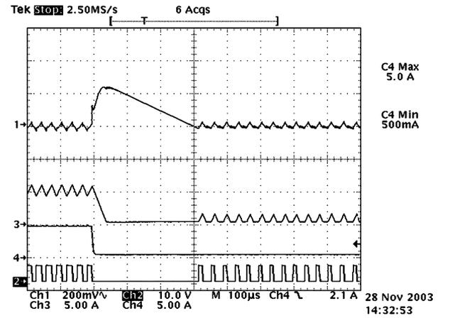
Fig. 10. Transient response of buck converter using second-order switching surface control. Load change from  $5 \text{ A}$  ( $2.4 \Omega$ ) to  $0.5 \text{ A}$  ( $24 \Omega$ ). [Ch1:  $v_C$  ( $200 \text{ mV/div}$ ), Ch2:  $v_g$  ( $10 \text{ V/div}$ ), Ch3:  $i_L$  ( $5 \text{ A/div}$ ), Ch4:  $i_o$  ( $5 \text{ A/div}$ )] (Timebase:  $100 \mu\text{s/div}$ .)
