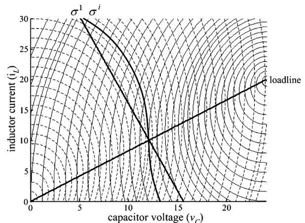
Fig. 2. State trajectory families of buck converter with  $\sigma^1$  and  $\sigma^i$ . (Solid line: on-trajectories, dotted line: off-trajectories.)
