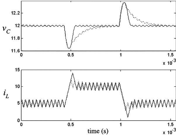
Fig. 7. Transient response of  $R$  from  $2.4 \Omega$  to  $1.2 \Omega$  and vice versa. (Solid line:  $\sigma^2$ , dotted line:  $\sigma^1$ ).
