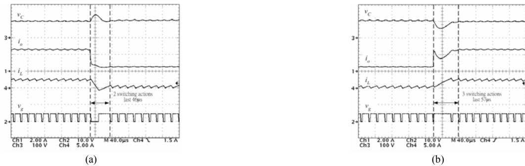
Fig. 11 Transient responses under load changes. (a) Rated load to 20% load. (b) 20% load to rated load. [Ch1: i_o (2 A/div), Ch2: v_g (10 V/div), Ch3: v_c (100 V/div), Ch4: i_L (5 A/div), timebase: 40µs/div].
