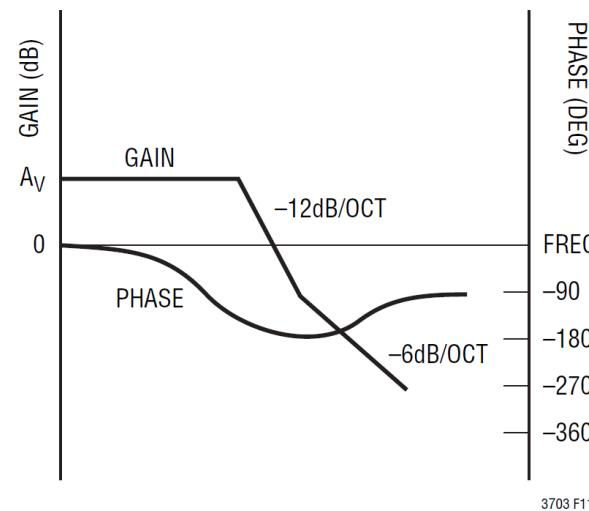
Figure 11. Transfer Function of Buck Modulator
